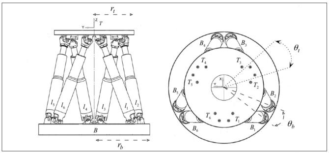
Figure 1: Kinematic configuration of the SP.
