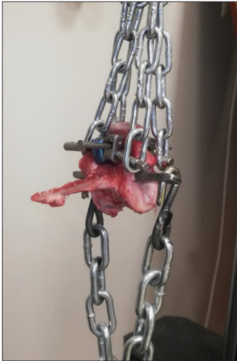
Figure 3: The instrumented vertebra was mounted to the upper and lower parts of the testing machine.
