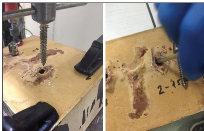
Figure 4: The primary screw pullout.
