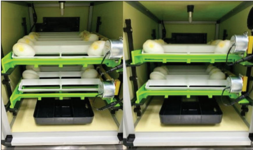
Figure 1: The arrangement of special pathogen-free (SPF) eggs within the incubator. The pointed edges of SPF eggs project downwards.
