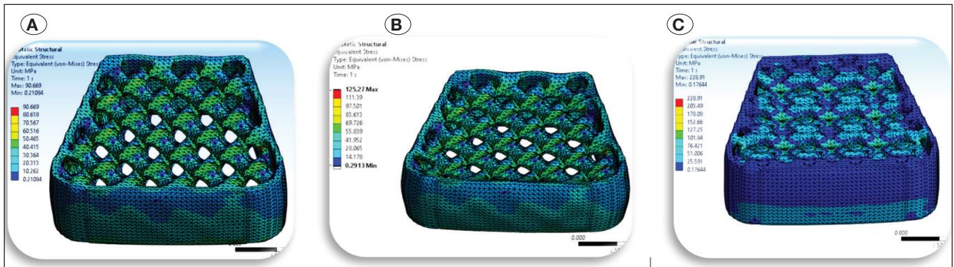
Figure 8: Maximum von Mises stress and its distribution obtained from the analysis.
