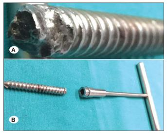
Figure 1: A) Shaping the broken screw head with the help of a high-speed drill. B) Compatibility of the removed broken screw with the extractor
