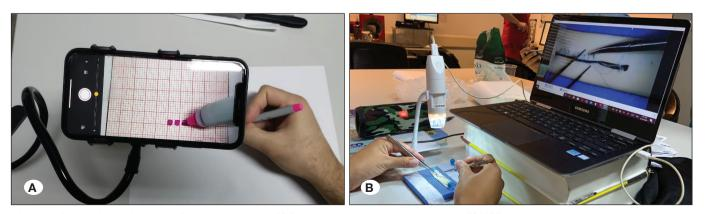
Figure 2: Alternative "microscope" imaging devices: A) Smartphone attached to a support. B) USB microscope connected to a personal computer.
