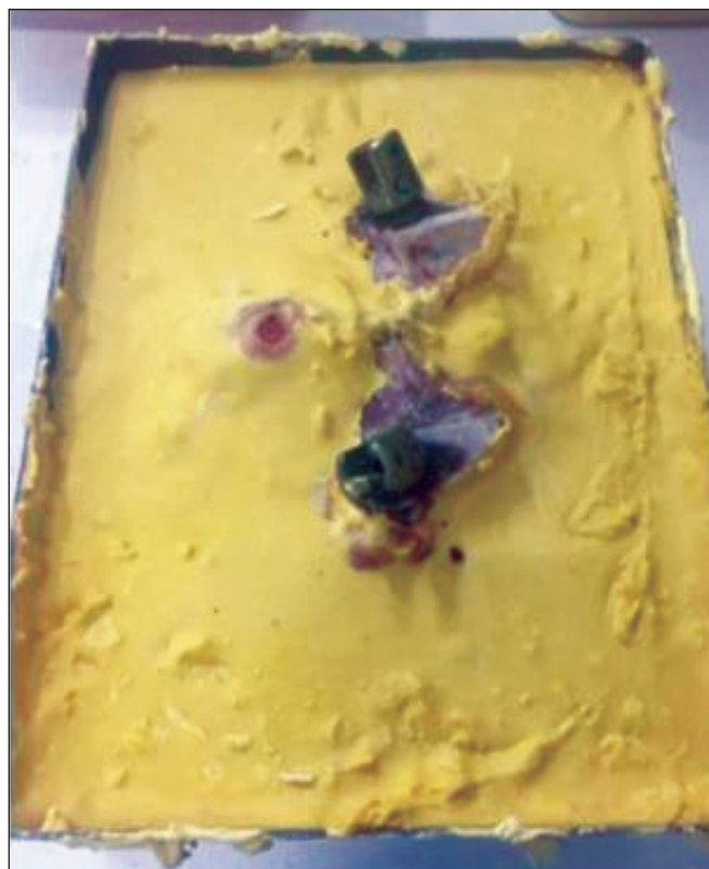
Figure 2: The anterior side of the vertebra buried in the cement with pedicles facing upward.
