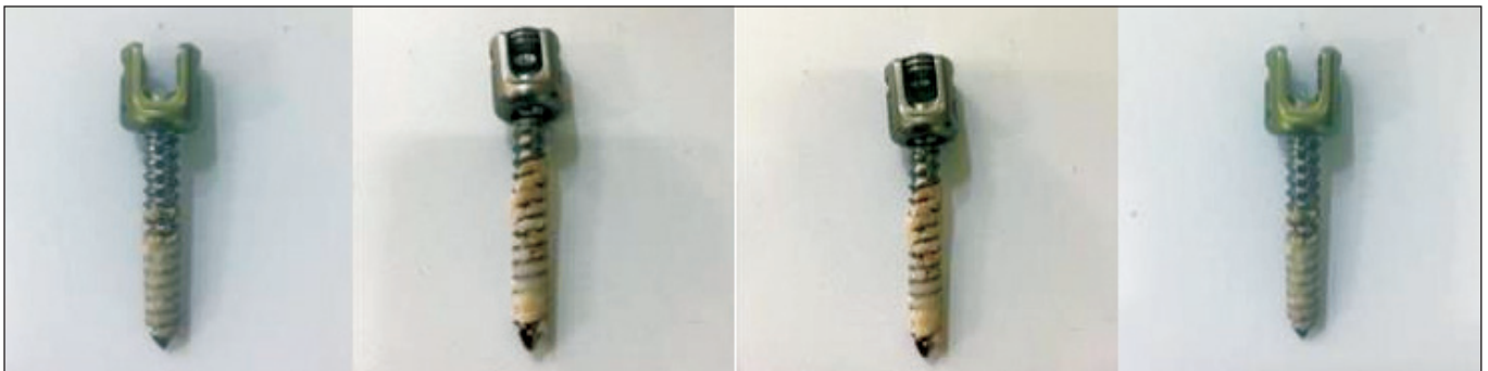
Figure 6: Screw samples after the second pullout tests were completed.
