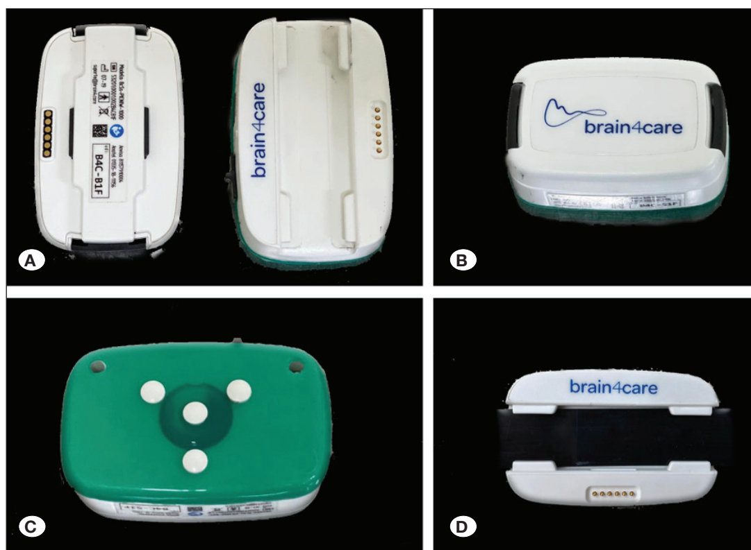
Figure 1: Picture for illustration of the sensor. A) On the left, the external battery unit for the sensor, which serves to recharge and extend battery life for prolonged usage, is on the right, the sensor, without a headband attached. B) Outer surface (no contact with patients) of external battery unit and sensor, connected. C) Inner, soft surface of the sensor, that is in contact with the patient's head. D) Sensor unit, with headband, attached.
